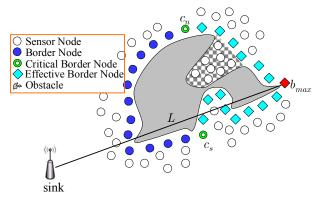
Fig. 3: An example of the farthest, critical, and effective border nodes.
