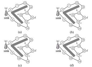
Fig. 1: An example of ping-pong effect in [4]. The number in each node represents the weight cost of that node. Node a changes its weight cost twice as shown from (a) to (d).
