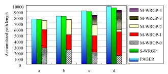
Four distributions of various numbers of obstacles ranging from two to five Fig. 11: Performance study of accumulated path length by varying the number of obstacles. The proposed M-WRGP significantly outperforms PAGER and S-WRGP in all cases.
