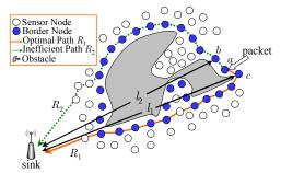
Fig. 2: The WRGP constructs an efficient route  $R_1$  while PAGER [4] and construct an inefficient route  $R_2$ .
