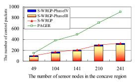
Fig. 8: Comparison of PAGER and S-WRGP in terms of the control overhead in the environment shown in Fig. 6(a).
