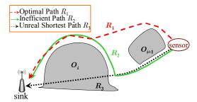
Fig. 4: An example that *S*-*WRGP* results in an inefficient route in the environment that contains multiple obstacles.
