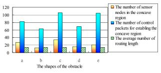
Fig. 7: The performances of S-WRGP examined in various shapes of the obstacle. Different shapes of the obstacle result in different numbers of sensors in the concave region and hence cause different control overheads.
